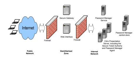
This diagram shows deployment E, using Password Manager and the Secure Gateway
