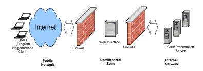
This diagram shows Sample Deployment D using SSL Relay and the Web Interface
