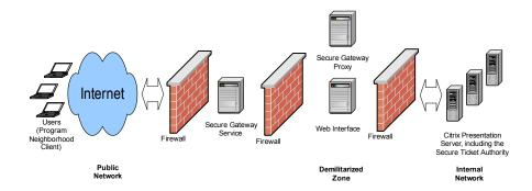
This diagram shows Sample Deployment C, which uses Secure Gateway (double hop) and IPSec
