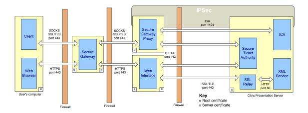
This diagram shows a detailed view of Sample Deployment C
