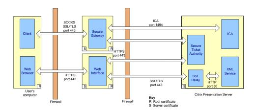
This diagram shows a detailed view of Sample Deployment B.1, which uses SSL Relay
