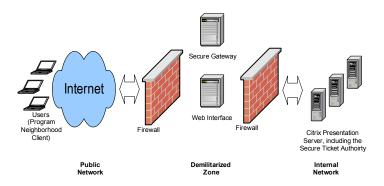
This diagram shows Sample Deployment B using the Secure Gateway
